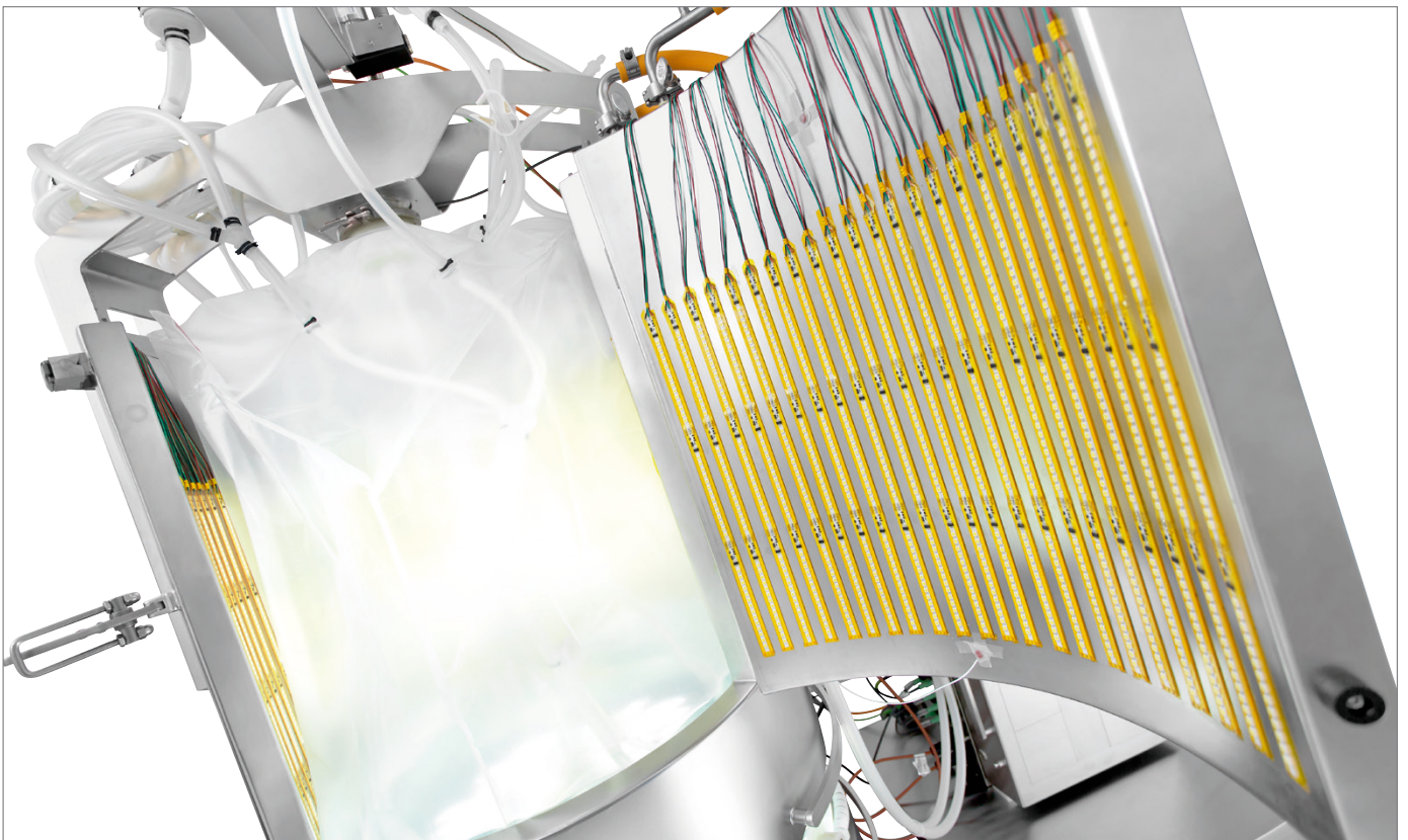
The customized bioreactor for Photoautotrophic Organisms is equipped with 5000 LEDs on the inside of the vessel to provide the essential light energy required for moss growth.
