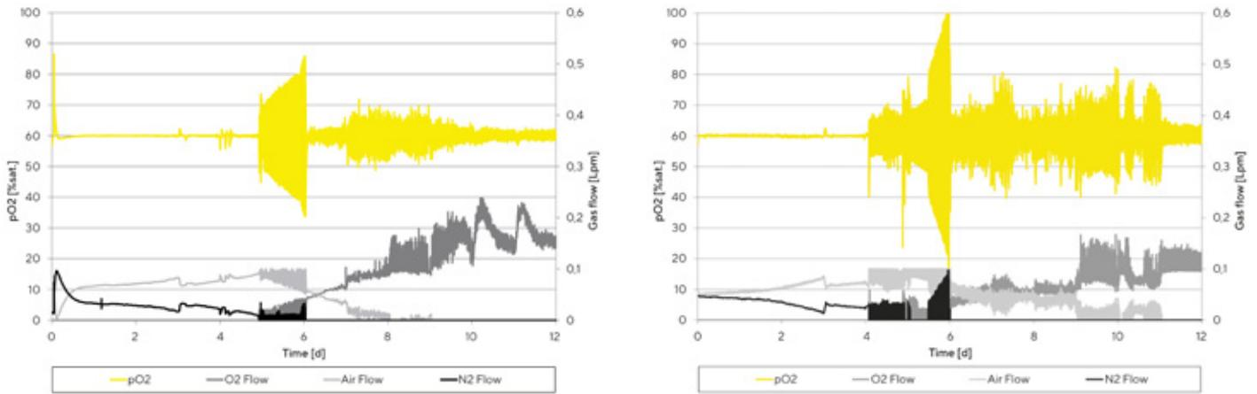
Figure 2: pO<sub>2</sub> and gassing trend – Univessel® Glass 5 L – micro sparger – Biostat® B-DCU (left) Biostat® B (right)
