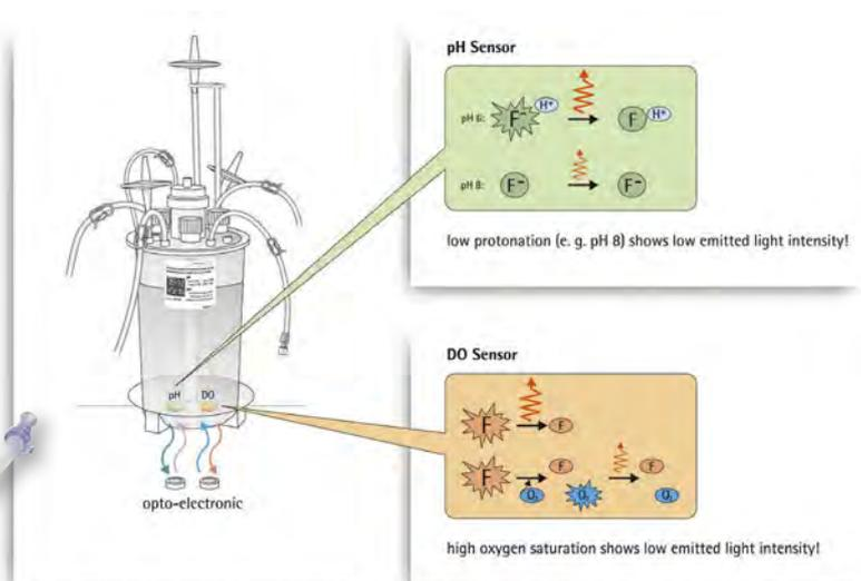
**Fig. 2: Functional Diagram of the UniVessel's Optical pH and DO Sensors**
