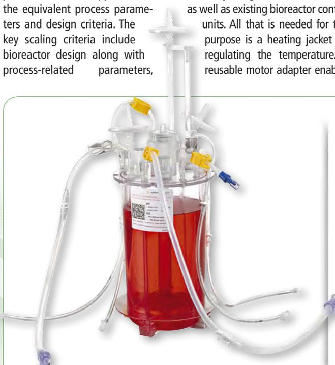
**Fig. 1: The UniVessel SU is a novel, single-use culture vessel specially designed for process development.**
